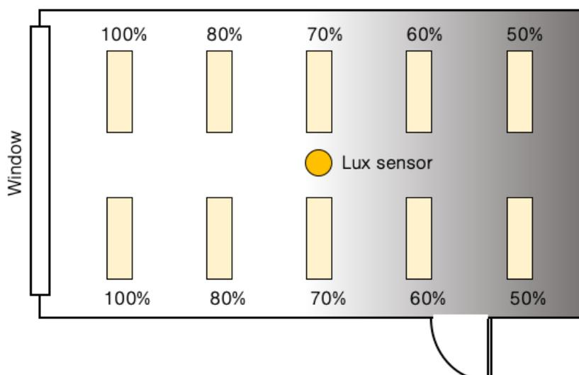
Each luminaire in a Casambi network can have its own daylight gain defined if desired. As standard the Daylight gain for luminaires is set to 100%.
